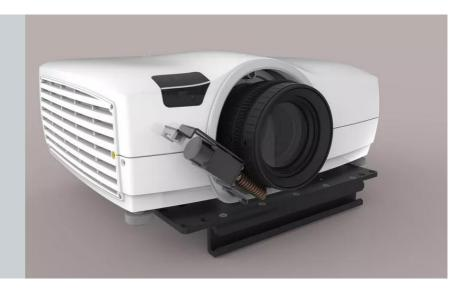
The F50 motorized iris kit is a complete solution that includes the F50 lens support. The stepper motor offers an accurate and repeatable iris adjustment. Power supply and communication is managed by the included USB cable. The F50 projector automatically detects the Iris Kit and enables iris control from the GUI.
