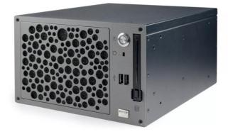
Barco's TransForm N 2-channel Output Node is a powerful PC-based network graphics processor. It is used in networked visualization environments and can display encoded streams coming from a Gbit Ethernet/IP network. The decoding blocks support MPEG-2, MPEG-4 and H-264 software decoding. Furthermore, the display controller also has a high-end graphics card to perform rendering operations as requested by clients in the network.
