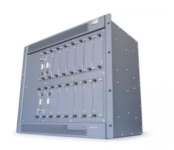
The TransForm XDS-400 is a multi-channel video processor for collaboration on large four- channel displays. It enables you to display up to six 2D, 3D and 3D stereo sources simultaneously on any type of display canvas - not just Barco systems.
