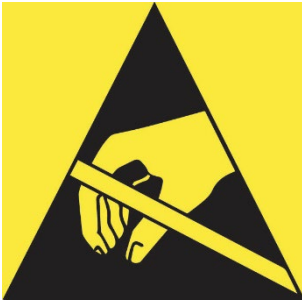
Figure 1 : ESD Susceptibility Symbol: to indicate packages containing electrostatic sensitive devices or to identify a device or a connector that has not been tested for immunity to electrostatic discharge.
