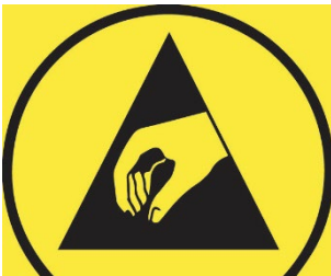
Figure 2 : ESD Protective Symbol: to indicate the primary function of the packaging regarding electrostatic protection.
