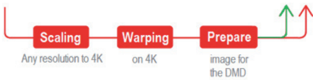
Figure 1. Conventional sequential processing steps in a projector
