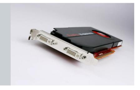
The MXRT-5450 is a high-performance PCIe display controller featuring AMD FirePro  $^{TM}$  3D technology for leading-edge performance, flexibility and reliability. The board supports DirectX and OpenGL and is compatible with Microsoft Windows® XP and Windows® 7.
