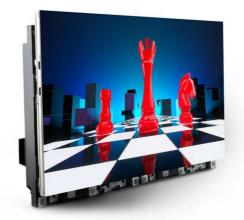
TruePix TP1.9 is Barco's new flagship indoor high-resolution LED platform. The 27.5" inch tiles, with a 16:9 aspect ratio, have a pixel pitch of 1.9 mm. TruePix is designed for control room, corporate and broadcast visualization applications and supports both environments exposed to ambient light and controlled lighting environments.
