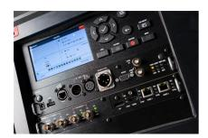
All new Pulse electronics have been designed to process 4K with  ${\rm HDMI}^{\rm TM}$  2.0a and HDCP 2.2 and the optical engine utilises the very latest 0.9" DMD DLP chipset, delivering 5,120 x 2,160 pixels to screen.Njord CS also features HDR, motorised lenses and Barco's unique RealColor processing, enables simple and accurate calibration to any desired color standard or white point.
