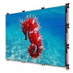
The award-winning Barco UniSee® platform has revolutionized nearly seamless LCD video walls and is a huge step forward in terms of image quality, installation precision, ease-of-servicing and reliability. Barco UniSee 500, offering typical brightness levels of 500 cd/m<sup>2</sup>, was designed for use in environments with controlled ambient lighting conditions. It complements the high-brightness Barco UniSee which is applicable in virtually every environment.
