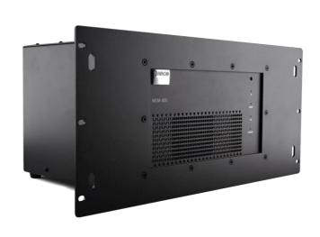
The MCM-400 is an external hardware component that allows geometry correction, color correction, and electronic blending on Barco's Galaxy 4K series projectors. By using a real-time on-screen user interface, the MCM-400 helps achieve the performance known from Barco's higher end simulation projectors. In this way, this box enables several multi-channel configurations with multiple 4K projectors.
