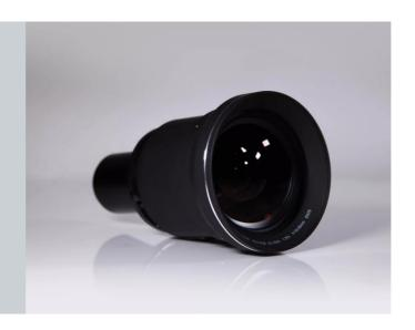
The EN76 lenses are designed specifically to maximize brightness, eliminate dust contamination, and to withstand motion and vibration through an improved barrel design. The lens consists of 20 glass elements with different coatings for the most demanding high-resolution performance, as well as being optimized for night vision and IR transmission. Additionally, to seal off unwanted air flow through the projector's front, through the grooves along the lens, a dust sealing has been designed.
