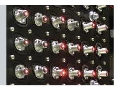
Barco's LDAT<sup>TM</sup> marks reference patterns to effectively align display channels. The LDAT<sup>TM</sup> provides a solution for up to 30 dedicated laser light sources which can be independently directed to points on the screen. Multiple arrays are used to mark a complete multi-channel system.
