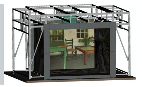
Virtual reality cave environments are typically custom-made system, answering exactly to the customer's specific needs. With the S4 Cave, Barco has bundled many typical requirements and developed a standardized environment. In this way, we can offer a very comprehensive system that answers the typical VR market demands for an attractive price point.
