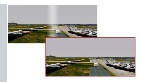
Multi-Channel setups of light-valve projectors lead to brighter overlap zones.Barco's standard Electronic Soft Edge Matching technology allows you to adjust edge blending to uniform level.
