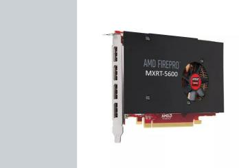
With the high-performance MXRT-5600 display controller, you can drive up to four monitors with just one PCIe slot. This makes it a perfect match for PACS workstations combining two diagnostic displays with additional displays for patient lists or 3D viewing applications. The MXRT-5600 is compatible with the DisplayPort interface standard, which assures easy installation and ultra-fast and reliable data transfers.
