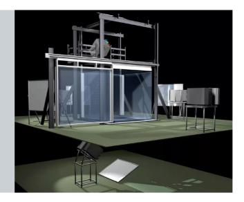
Barco's I-Space is a multi-sided, cubic immersive environment that surrounds the user completely with virtual imagery. It consists of three to six walls, according to the user's requirements.
