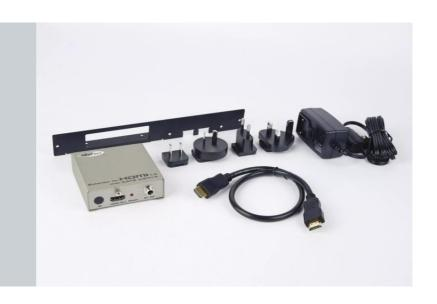
Barco's HDBaseTTM option is a receiver module for transmitting high-quality, uncompressed video signals through a single network (CAT6) cable. It is a cost-efficient solution that supports resolutions up to WUXGA for a distance of up to 100 meters (330 feet).
